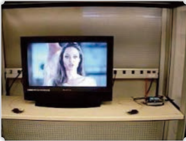
圖 2 Demonstration of wireless uncompressed HDMI video streaming, using single-chip 60GHz 90nm CMOS transceiver. [2]
