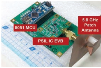
圖 6 A 5.8GHz Phase- and Self-Injection-Locked CMOS Radar Sensor Chip for Vital Sign Detector [6] Miniaturization Gas Sensing
