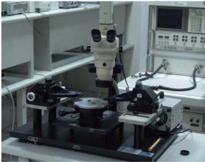
On-wafer measurement system with HP8510c and CASCADE probe station
