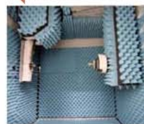
Millimeter-wave chamber (1.3x1.3x1.5 m 3 )
