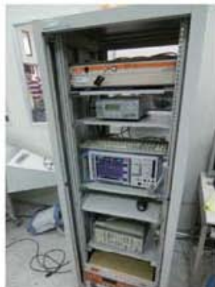
(top to bottom) Probe Laser Interface, Boonton 4231, ROHDE&SCHWARZ FSP40, DC Power Supply AR Model 20ST 1G18A
