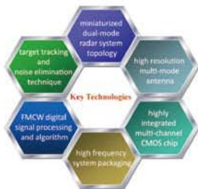
Field of view and key technologies of the dual-mode millimeter-wave vehicle radar system
