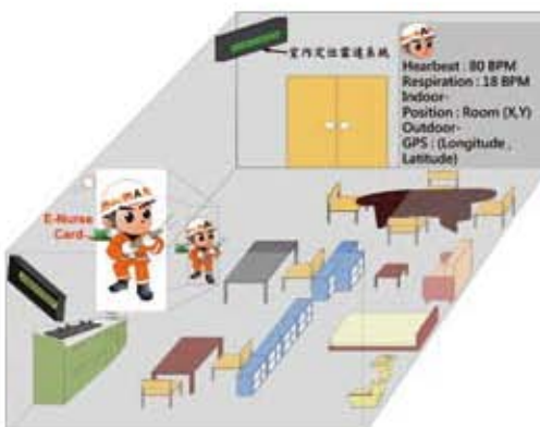
Fig. 3 Emergency E-nurse system: Cardiopulmonary Detection and Wireless Positioning
